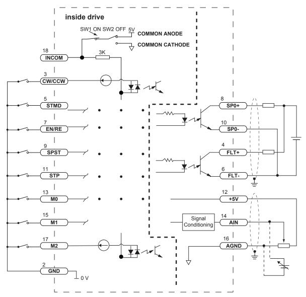
Connecting to control IO with internal Sinking Outputs
