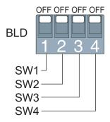
For RS485 version, SW4 is "ON" that means there is a 120 ohm termination resistor across the TX+ and TX- terminals. SW3 is reserved.
