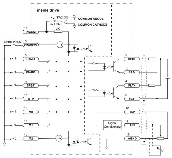
Connecting to control IO with internal Sourcing Outputs
