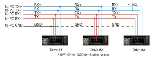
NOTE: If the PC does not have an RS-485 serial port, a converter is required. You can contact MOONS' to buy a USB to RS-485 converter.
