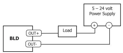
Connecting a Sinking Output
