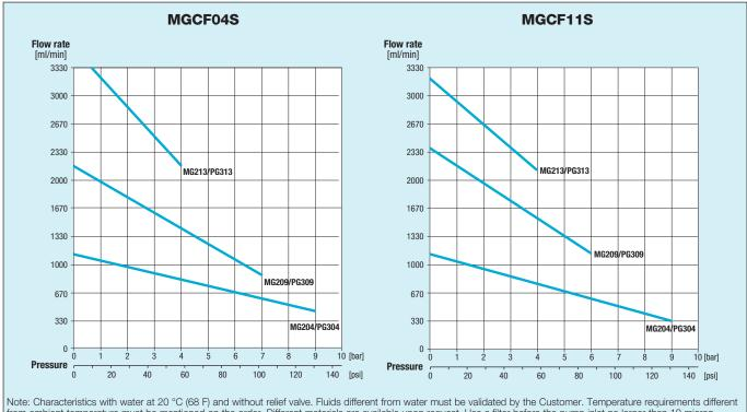
Note: Characteristics with water at 20 °C (68 F) and without relief valve. Fluids different from water must be validated by the Customer. Temperature requirements different from ambient temperature must be mentioned on the order. Different materials are available upon request. Use a filter before the pump inlet no larger than 10 micron
